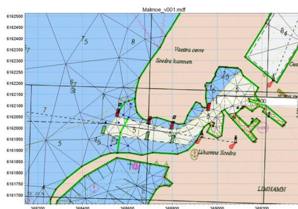
Example of Flexible Mesh generated for a flushing study in Port of Malmö, Sweden. The background image is from MIKE C-Map which enables extraction of land contours and water depths from digitized Admiralty Charts provided by Jeppesen Norway
