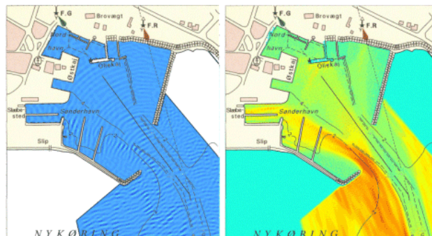
Output from MIKE 21 BW 2DH. The panel to the left shows a map of the instantaneous surface elevation. The right panel shows the map of the corresponding wave disturbance coefficients. Nykøbing Mors harbour, Denmark
